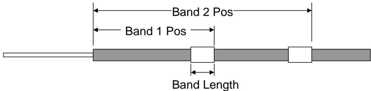
After positioning each band, the machine uses Blockwise's 6-jaw precrimper to form the band into a hexagonal shape that holds it firmly in position for swaging.
