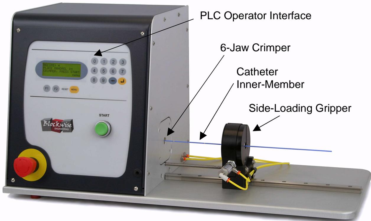
The band positioner / precrimper model PMC uses a simple, reliable, mechanical approach to positioning bands, with no optical sensors or vision systems. The PLC control software can be set up by a novice in just a few minutes.
